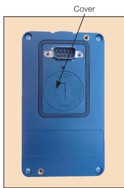
Figure 28: Keypad battery cover to access battery
