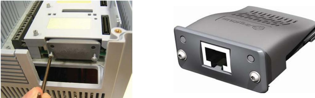
**Figure 1:** Anybus-CC Installation
