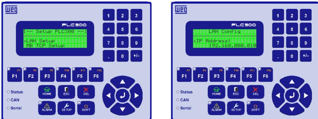
**Figure 5:** PLC300 LAN Setup Configuration
